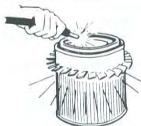
Compressed air cleaning method
