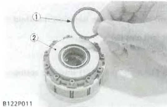
(1) Commutator Seal (2) Commutator Cover
